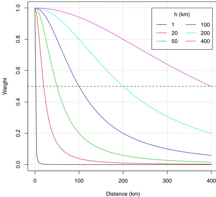
Figure 2: Different shapes of the weighting function according to the weight distance  $h$  (parameter *wc* of the homogen function).
